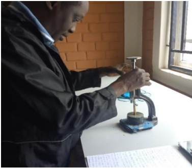
Plate 1. Performing consistency /setting time test
